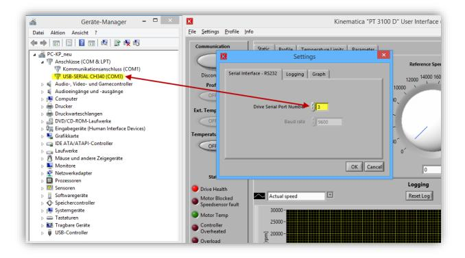
17. The dispersing device is connected with the software by clicking on **Communication**.
